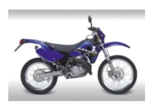
line with the taste of its users. With the 125, 250 and 300 cc bikes, this 2-stroke single cylinder with a Deltabox chassis made with elliptic profile Cr-Mo tubes, has had its brakes reinforced, especially the front brake, whose disk is now 240 mm, with a 4-piston self-centering vice. The rear disk is still 200 mm.
