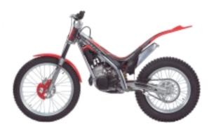
Mo). Equipped with a Marzocchi 140 mm hydraulic fork in front and a Boge 155 mm hydraulic rear racing fork, this small frame becomes a replica of her big sisters, offering the same features, but of course in mini size.
